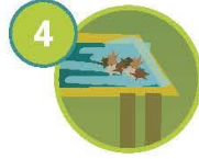
4 Flat roof with standing water
